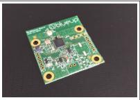
BlueBeacon 06/UFL is a low-profile single-board BLE beacon, with UFL connector for external antenna.
