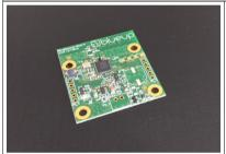
BlueBeacon 06/ANT is a low-profile single-board BLE beacon, with integrated omnidirectional PCB antenna.
